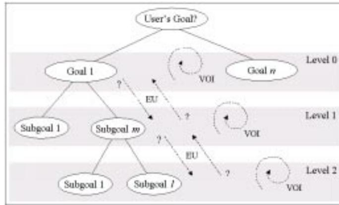
**Figure 1.** Schematized view of an overall model for guiding diagnosis of goals via Bayesian inference, computation of value of information (VOI), and expected utility analysis (EU) for navigation between levels of detail for progression and backtracking in conversation.
